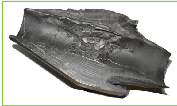
Breakdown traces on the field steering body of a 110 kV cable
